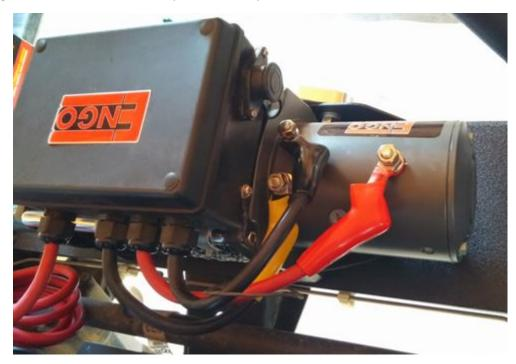
6. Screw the thin black cable from the solenoid box and the long negative battery cable into the black screw port at the bottom of the winch using a 14mm socket or wrench.
