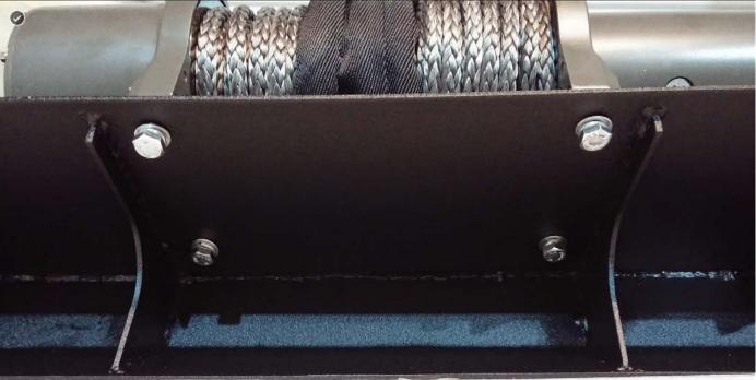
3. Mount the bumper or winch plate to the vehicle using instructions provided by the winch plate or bumper manufacturer and feed the winch cable end loop through the fairlead. Next, attach the cable hook to the cable loop.
