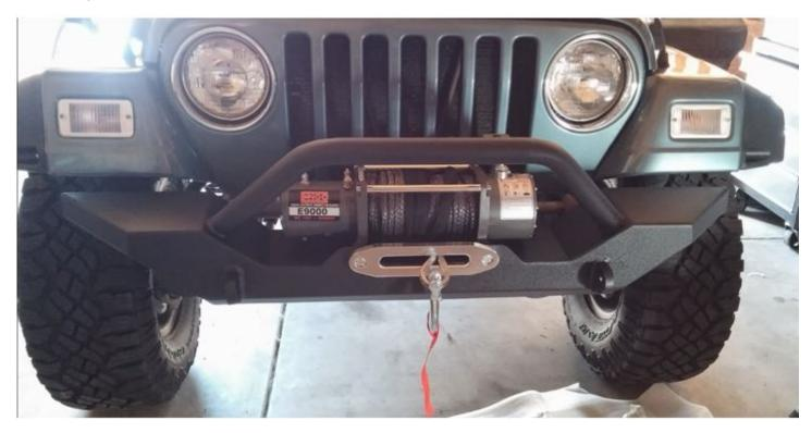
4. Mount the solenoid box. Make sure the screws on the solenoid box clamp are loosened all of the way before installing. Hook the front of the solenoid bracket onto the upper front bar of the winch and then clamp it onto to the upper rear bar. Once seated properly tighten the screws in the back of the bracket with a Phillips head screwdriver.
