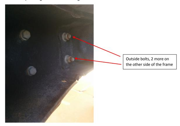
3. Install the bracket to the frame. Mount with the horizontal holes against the front of the vehicle. Use a bolt, flat washer and then a flat washer and lock nut on the back side. Tighten both bolts down using the 18 mm socket on the head side and the 19 mm wrench on the nut. Use the mallet to slightly angle the top of the bracket in towards the frame.
