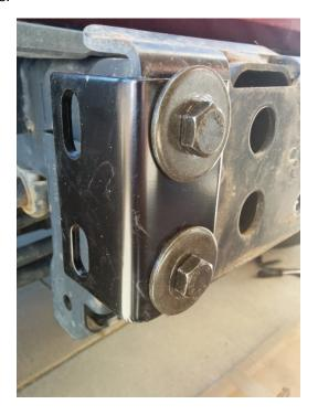
4. Place the bumper onto the brackets by sliding the bottom of the bumper mount onto the top corner of the frame mount. It will be tight but continue to apply pressure downward and slide it into place.
