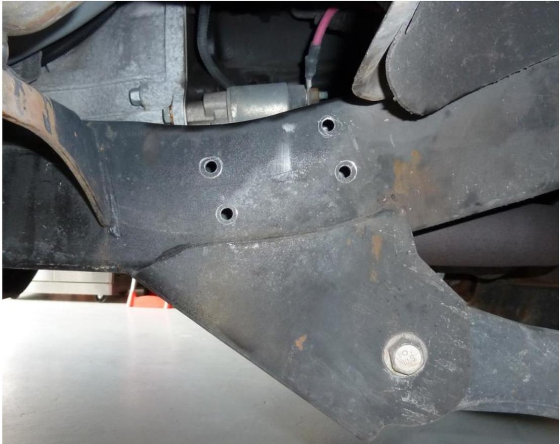
5. Re-position guard against frame and align mounting bracket holes with holes in frame. Install self-tapping bolts in all holes. Do not tighten bolts completely until all bolts are started. Once all bolts are in place, tighten all bolts securely. *Alternatively, you may pre-tap all holes with the guard out of the way. Be careful not to damage threads when removing bolts.*
