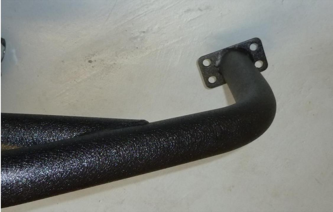
The rear bracket of each guard is mounted straight.
