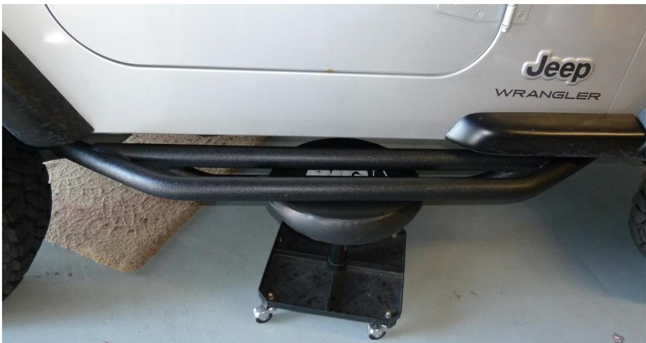
2. Check placement of mounting brackets to ensure they are not resting on, or coming in contact with other brackets or components, and do not extend above or below frame.
