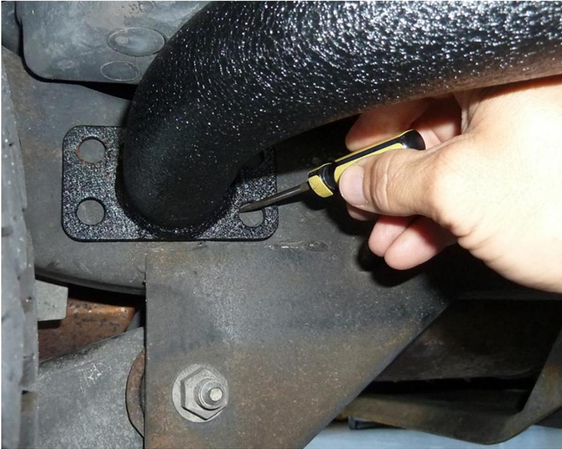
4. After marking all holes, move the guard out of the way. Center punch all marked locations. To ensure precise placement, drill pilot holes at all locations using smaller diameter bit. *Check for hazards or obstructions before drilling.* After all pilot holes are drilled; drill all holes with 5/16" bit.
