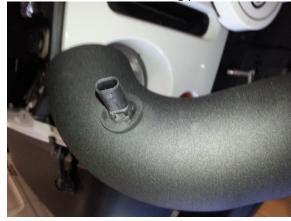
**Step 12:** Install the supplied coupler to on the intake and the throttle body and secure it on the vehicle.
