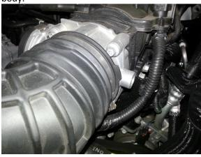
**Step 5:**Pull the entire intake assembly up and away from the vehicle.
