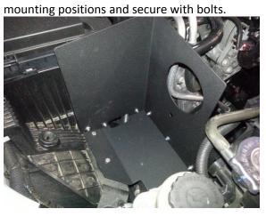
**Step 10:** Add the supplied rubber gaskets to the top of the heat shield and in hole for the intake.
