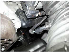
**Step 2:** Slide the PCV hose off of the factory air box.
