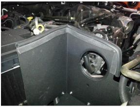
**Step 11:**Remove of OEM IAT sensor and transfer it over to the new intake tube noting position.
