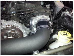
**Step 13:** Reinstall the factory PCV hose onto the new intake tube and secure with new clamp.
