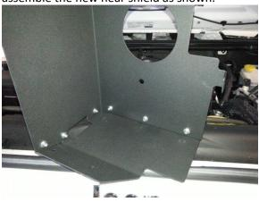
**Step 7:** Add the supplied screws and spacers to the heat shield for mounting in the factory position.
