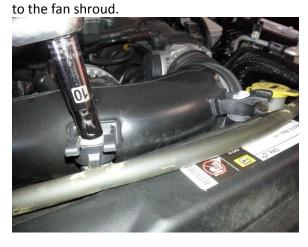
**Step 4:**Using a flathead screwdriver, remove the hose clamp holding the intake tube to the throttle body.
