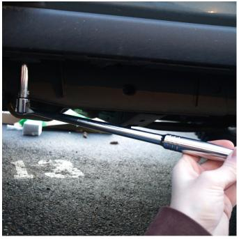
2. Insert the bolts into the rails. Due to the thickness of the coating the washers may not want to fit. You can motivate them by hitting them with the side of the breaker bar (or a hammer).
