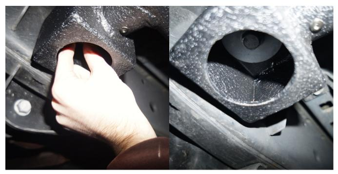
5. Torque each of the bolts to factory spec (35 ft\*lbs) in an in several intermittent steps while alternating between bolts. Do not torque one bolt fully then torque the other fully. **Warning:** These bolts are tapered; if you crank one down all the way first and then attempt the other you may strip out the threads.
