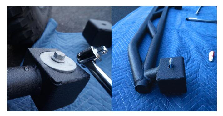
3. Apply some blue (semi-permanent) thread locker to the threads.
