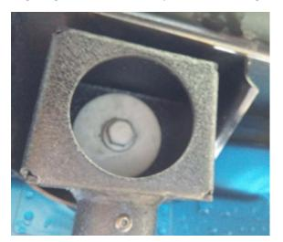
9. Leave the bolts loose until all 3 are in place so you can adjust the sliders to line up all of the holes.
