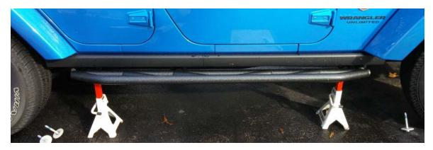
8. Following the instructions, put the blue Loctite on the bolts. Slide the bolts back into place through the mounting holes in the sliders. Finger tighten the bolts into place and then tighten a few turns with the wrench.
