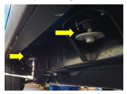
6. Use a pry bar to finish removing the bolts from the body insulators.
