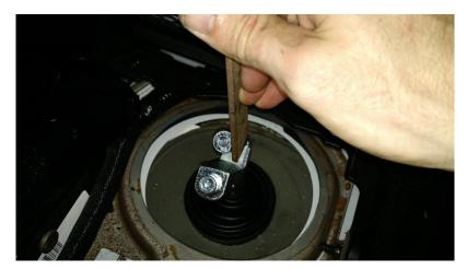
9. Reinstall the inner shift boot back down the shaft and on top of the extension. Push the folds of the boot down as far as possible. Reinstall square clip, outer boot/bezel, and shift knobs back in reverse order.
