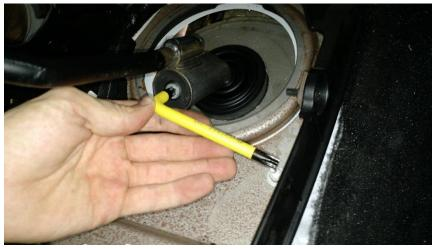
6. Install the extension onto the transmission stub. Try to slide it down all the way and remember lubrication is your friend. ☺
