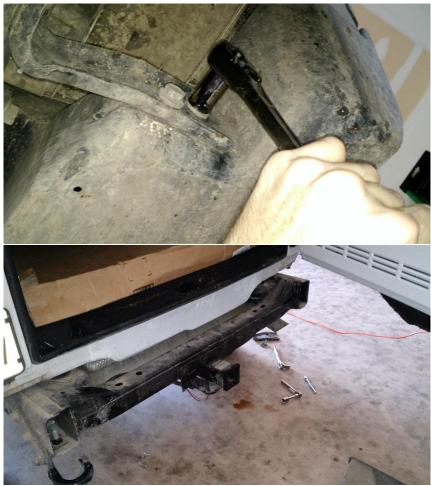
7. Using an 18mm socket, go around the entire body and loosen the big center stud bolts. Do not totally remove, just loosen to give you clearance when you jack up one side at a time. You'll need the extension on the rear most center nuts. On this 2014 4 door, there are ten body mounts all together: 2 in the front by the grill, 3 along each side of the frame (6 total), and 2 in the very rear by the muffler.
