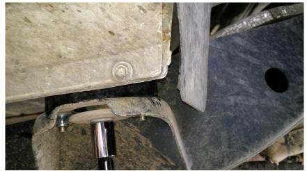
20. Reinstall the rear bumper using the supplied extension brackets and the original bolts. The center brackets top bolts are easier to hand tighten from the top, then tighten with a 16mm wrench from the bottom. Insert and tighten the each lower bolt for both center brackets using a 16mm wrench.
