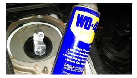
7. Apply thread locking compound and tighten the 8mm Allen head bolt with a 6mm Allen head wrench. Tighten the set screw with the 1/8" Allen wrench.
