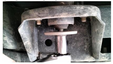
8. Starting on the driver side, remove the two stud nuts from each body mount using a 16mm socket. The front body mounts are upside down compared to the rest of the body mounts. You'll need the extension again for the rear most body mounts.
