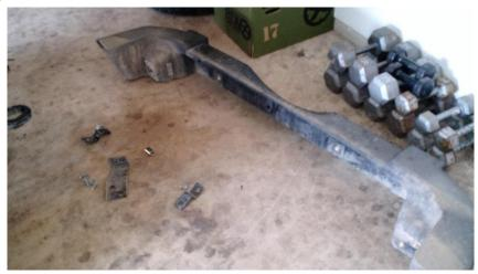
5. Using a 16mm wrench, remove the top and bottom bolts from the two inside brackets supporting the rear bumper.
