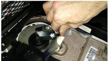
8. Install the shifter onto the extension using the T45 Torx wrench. Note: I needed to use a file (or use the grinder) on the flat side of the extension to get the shifter to fit down onto it.
