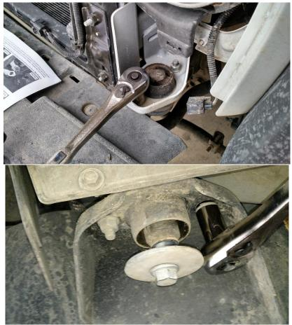
9. Remove all the center stud bolts from the same side, driver side, using an 18mm socket. If the bolts are dangling loose but you cannot remove, you may need to pry the bolts out. This is due to the little retainer clip used at the factory. The may have already rusted off too.
