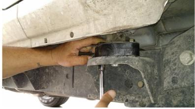
13. The blocks will go on the frame side of the body mount except for the front two mounts. These front two will be opposite, on the body side.
