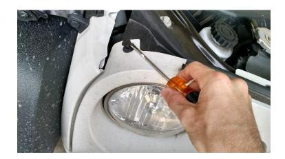
3. Disconnect the plugs to the parking lights on either side of the grill before totally removing from the vehicle.
