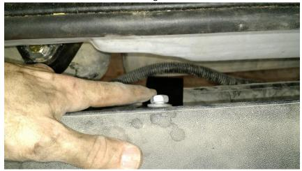
21. Use a 16mm socket to tighten the new side brackets using the original bolts.
