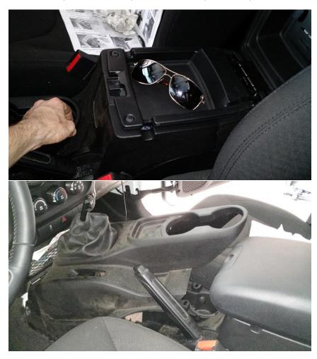
3. Once that's out of the way, unscrew the square clip holding the inner shift boot to the body.
