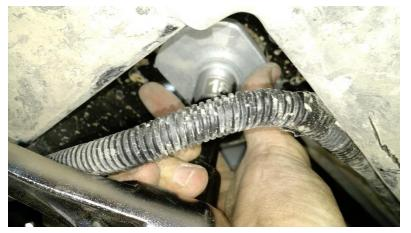
19. With all of the center stud bolts inserted and threaded by hand, lower the passenger side and remove the wood blocks. Tighten all the center stud bolts with an 18mm socket to 80 ft/lbs.
