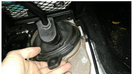
5. Remove the shifter with a T45 Torx wrench. Save the hardware for reinstallation on the extension.
