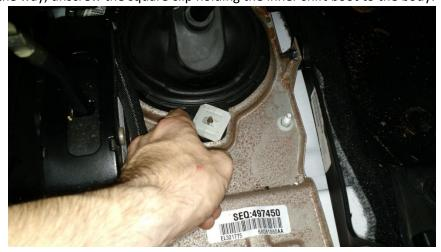
4. Pull the boot up from the back and slide it off of the shaft.
