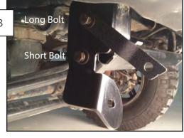
Insert a long 18mm bolt through the small bracket then into the top hole of the large bracket. Insert a short 18mm bolt into the bottom hole of the large bracket. Hand tighten bolts.
