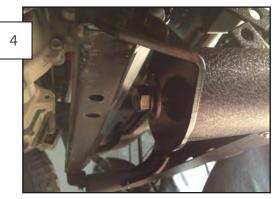
Move the bull bar into position and insert the two 19mm rear bolts
