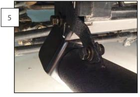
Insert the smallest bolt through the small bracket and bull bar top mount, then attach it with the supplied lock nut. Hold the bull bar in position and tighten down all hardware.
