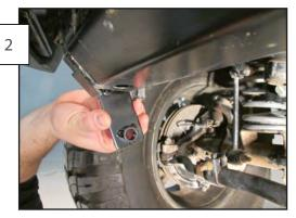
Insert a double nut plate into the opening on the bottom of the crash bar with the flat side facing the outside of the vehicle.
