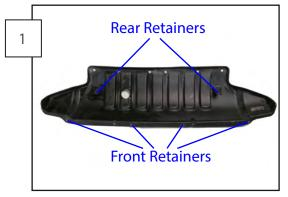
Remove the 4 front and 2 rear, plastic push pin, splash shield retainers.
