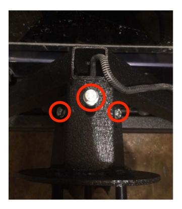
11. Bolt your spare tire onto your tire carrier and tighten the three lug nuts they give you with the kit. Your installation is now complete.
