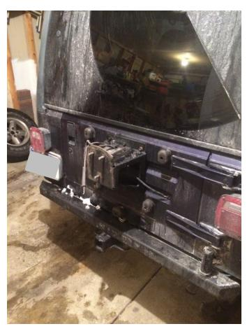
7. To remove the stock spare tire carrier you have three 13 mm bolts on the top of the carrier (Left) and two 13 mm bolts on the bottom (Right). Remove these five bolts and your tire carrier will come right off. Note: I put these bolts back in the tailgate so there wasn't any empty holes.
