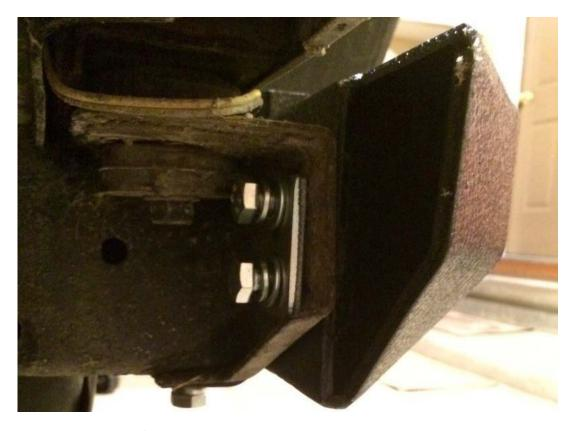
5. You can now take the two 7/16 bolts with a lock washer and a washer on each bolt. You may only use one hole. These bolts will bolt into the bottom of the frame, tighten these ones now. Once you get the bolts in you can snug up all of the other bolts on the bumper. The bumper install is completed and you can start with the carrier.
