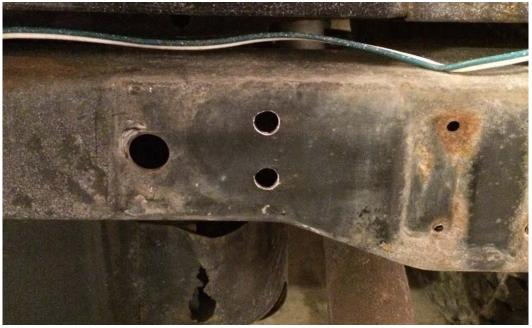
4. Now you can mount the bumper to the frame using the four backing plates and the 3/8 bolts with lock washers and washers on each bolt. Do not tighten the bolts just yet, leave them loose. Do this with all four sets of holes, two on each side of the frame.
