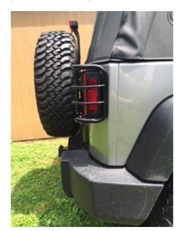
4. Finally, tighten all screws as you check for clearance on body and light assembly.
