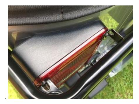
3. Insert final two screws making sure to add washer and grommet before installation.
