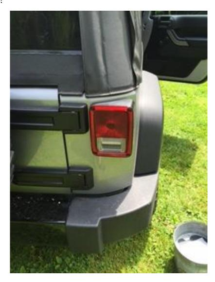
1. Unscrew stock screws from tail light assemblies.
