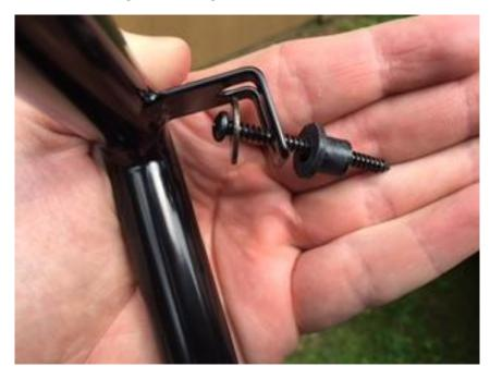
2. Attach two screws (opposite ends of tail light) as checking for alignment on tail light assembly and body of Jeep
