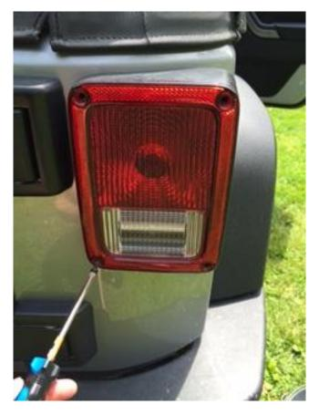
1. Attach tail light covers on tail lights with new screw, washer, and rubber grommet, only hand tight. Make sure rubber grommet is between tail light and tail light covers.
