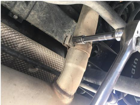
2. Once the clamp is adequately loose, I disconnected the hanger from the muffler on the drivers side of the Jeep (leave the passenger side attached for now). This freed up the muffler to move without falling once the muffler was removed from the mid pipe.
