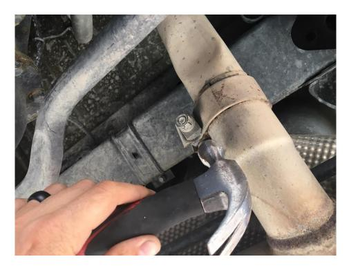
4. Once the muffler is disconnected from the mid pipe (again the WD-40 saved my life on this step), disconnect the passenger side hanger (you may have to use WD-40 on both hangers as well, depending on your Jeep and how corroded they are) and remove the muffler.
