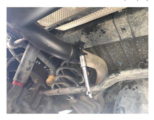
6. The last step is attach the tailpipe tips with the provided clamps and you are done!
