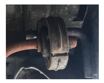
3. Once I had the nut loose, and the drivers side hanger disconnected I used a few shots of WD-40 to loosen the bond between the mid pipe and the original muffler, and then started tapping with my hammer to dislodge the OEM muffler from the mid pipe. I also used a 2lbs hammer to knock the original muffler off the mid pipe.
