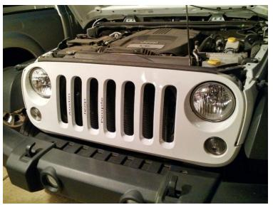
3. Start by using the flat head screwdriver to pop the six plastic retainer tabs located along the top of the grill. Then pull the bottom of the grill towards you to pop the retainer clips out.
