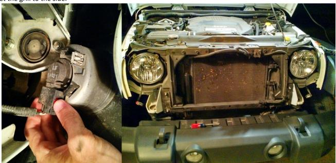
5. Use the T15 Torx driver to remove the four screws holding the headlight retainer ring in place.
