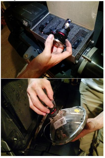
9. Move back to the front of the Jeep and plug the LED headlight into the wiring harness. *Note: My harness would not stay in very well and the red locking tab would not click forward. I used black electrical tape to secure.*
