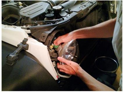
7. Remove the headlight bulb from the headlight assembly by twisting left until it unclips.
