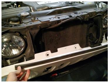
4. Next you'll undo the turn signal wiring harness by pulling the red locking tab, then disconnecting the harness. Set the grill to the side.
