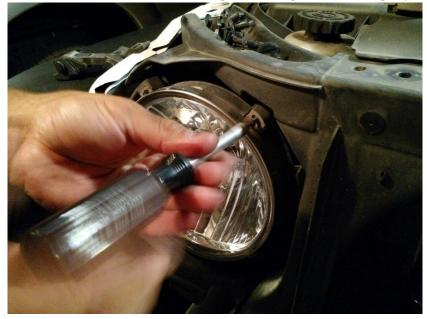
6. Set the retainer ring to the side and unclip the headlight bulb from the wiring harness. You'll have to push the red locking tab back in order to remove the clip.
