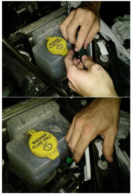
14. Finish up by reinstalling the grill. Reinstall the turn signal harnesses and lock the red locking clip. Push the bottom of the grill into the jeep until the retaining clips click in, then use the six black clips to secure the top of the grill.
