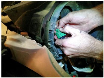
10. Fish the wires and ballast through the back up to the top of the engine bay and reinstall the headlight with the retainer ring and the four T15 Torx screws.
