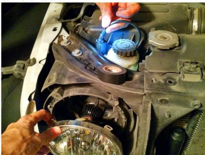
11. Grab the double sided sticky tape provided and use a knife to cut an appropriate size to fit on the back of the ballast.
