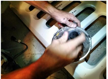
8. Remove one of the LED headlight bulbs from the box and insert into headlight housing. The wires should be sticking down when the headlight is vertical.
