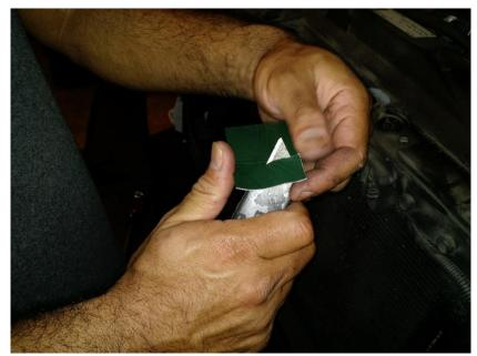
12. Find an appropriate spot to tape the ballast to and clean that spot and clean the back of the ballast to insure good adhesion. *Note: The passenger side was much easier to find a spot than the driver side. This might be different on earlier models or those with different intakes/filters.*
