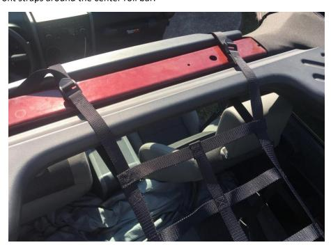
3. Take the other two straps and attach around the rear roll bar.
