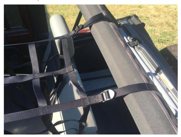
4. Attach all four left side straps to the roll bar.
