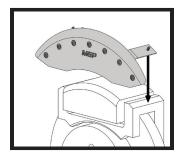
Place the caliper cover on the brake caliper. Cover should be centered across the front. Caliper cover bridges should be positioned against the brake caliper bracket.
