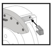
Slide the stainless steel clips over the bridges and caliper brackets and around the threaded studs to fasten the cover. Fit should be snug and secure.
