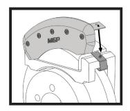
Place the cover over the caliper and position hole in bridge over the threaded stud and onto the clip (may require some force to pull second hole over stud).
