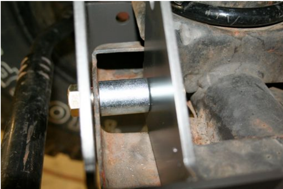
Detail view of track bar relocation bracket spacer installed
