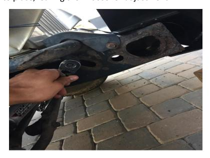
5. Install the (6) 19mm hex bolts into place, Again leaving them loose for adjustment Make sure the bumper is centered and then tighten all of the bolts.
