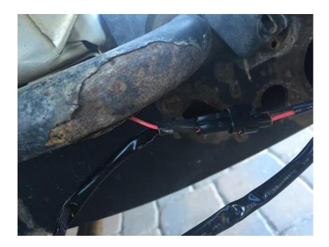
7. Cut the original fog lights wires and then connect the led red and black wire to the original blue and black fog lights wires then secure them with electrical tape.(Black-Black/Red-Blue)
