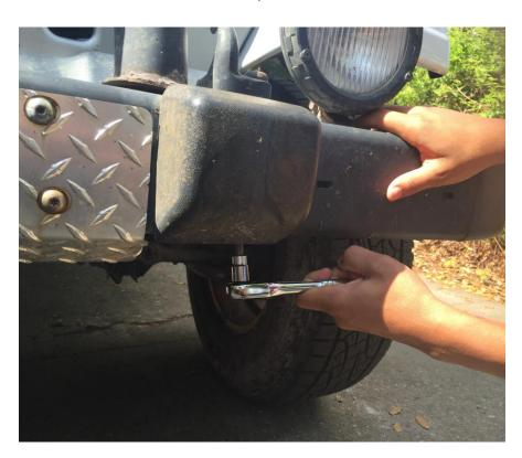
2. Remove the (4) remaining T-55 Torx bolts and pull/remove the Bumper. A buddy would be helpful.
