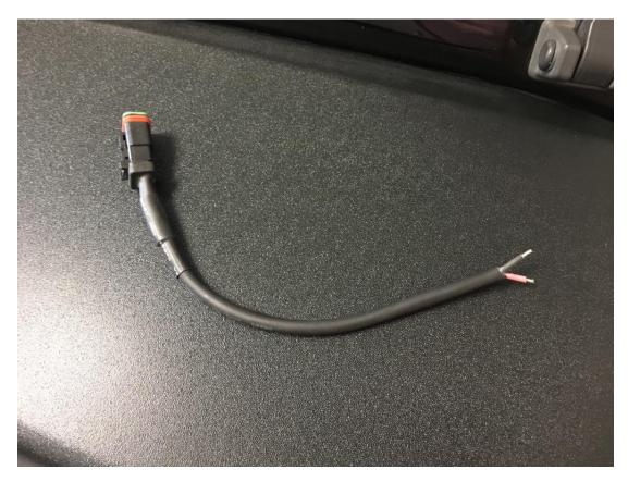
10. Connect wiring quick connects and route wires to engine compartment so as not to interfere with hood closure and secure wires as desired
