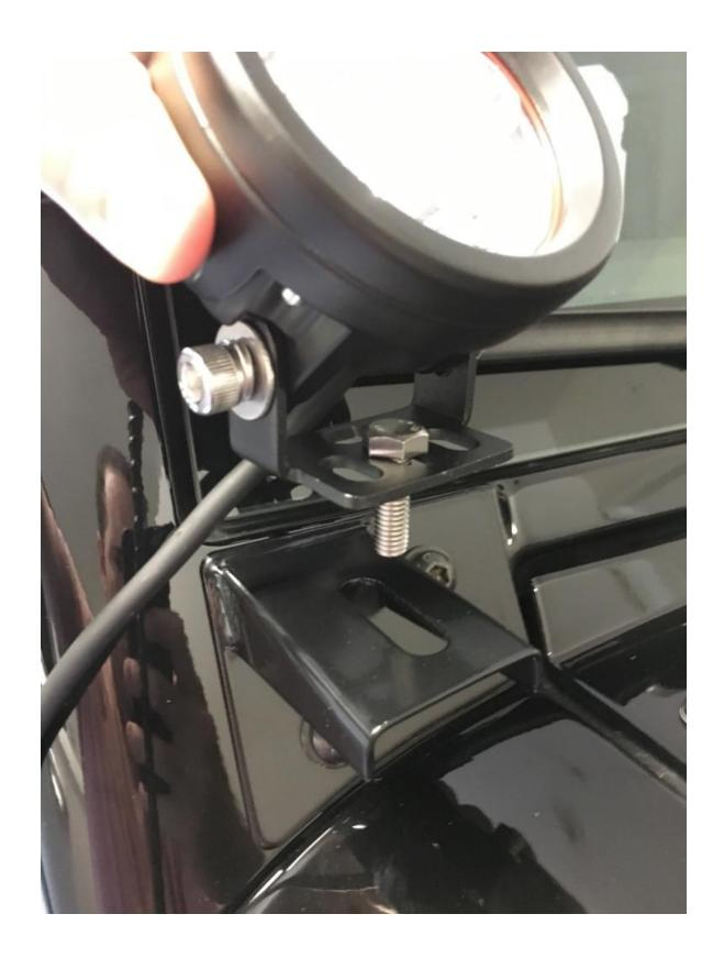
6. Install light bracket to mounting bracking using provided bolt, washer, and nyloc nut - snug up with ½" openended wrench on nyloc nut and crescent wrench on bolt paying attention not to over-tighten before
