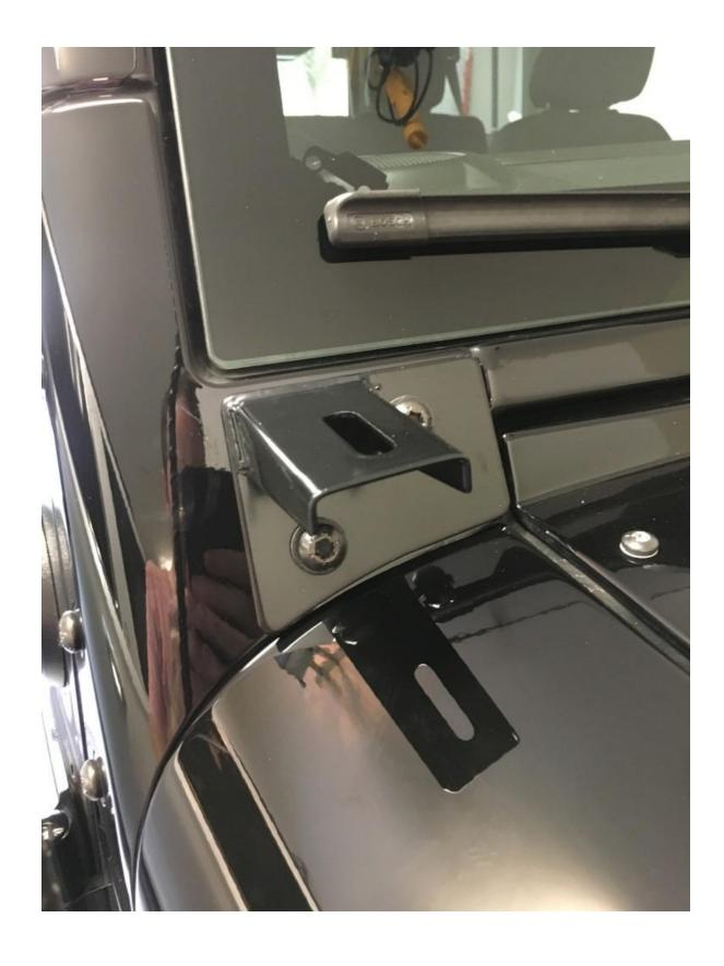
4. Remove fog lights from packaging and install brackets to lights with bolts, washers, and lock washers provided
