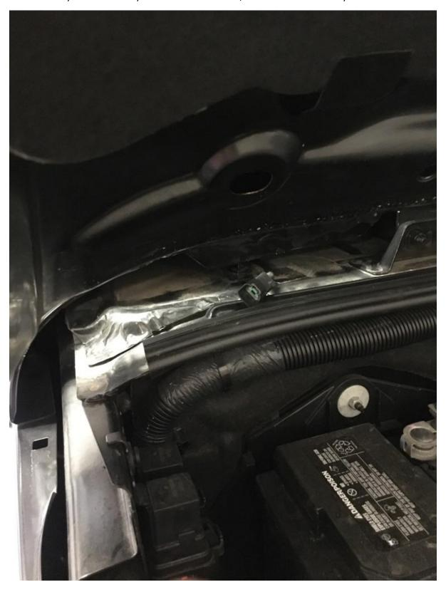
9. Wire included pigtail and quick connect male end to wiring harness (not included - see specific manufacturer's installation instructions)
