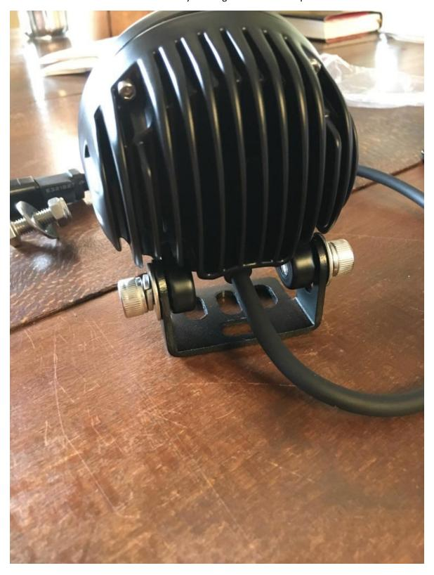
5. Tilt bracket on light and install bolt for installation to mounting bracket previously installed on Jeep
