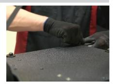
With the security cargo lid aligned and all bolts in place, tighten all of the hardware.
