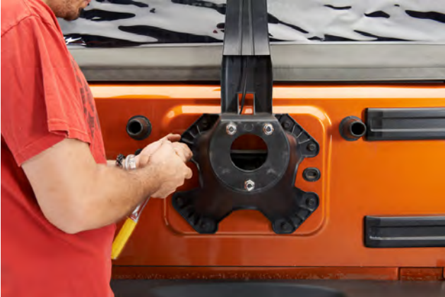
STEP 1 // Remove the rear tire and the (8) 13mm bolts holding the tire carrier to the tailgate.
