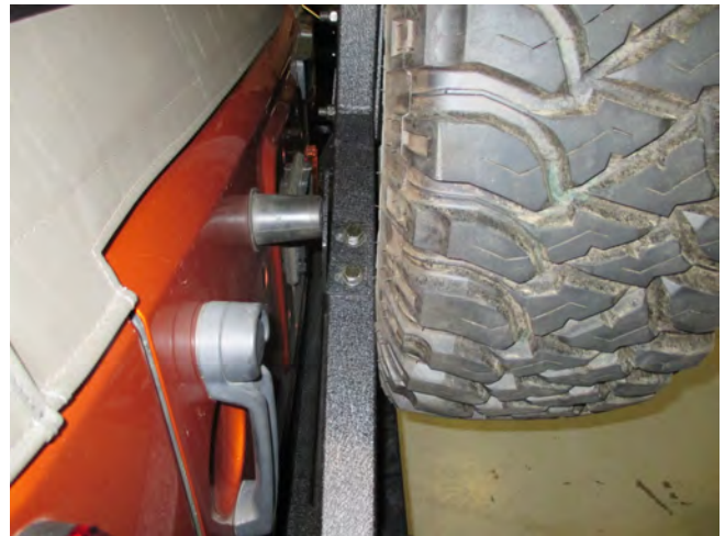
STEP 15 // Torque the spare tire lug nuts to the manufactures specified torque spec.
