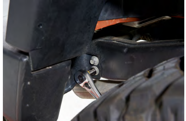
STEP 3 // Remove the (4) 15mm bolts securing the rear bumper.
