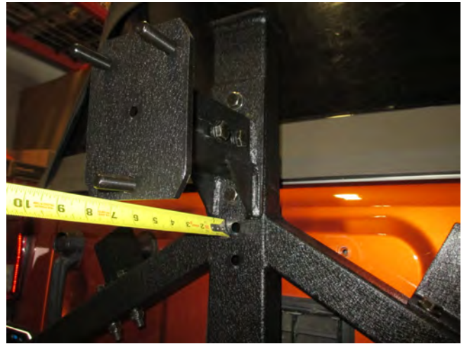
STEP 14 // Subtract a half inch from the previous measurement, and set the carrier to the new measurement. This insures the tire is against the carrier.
