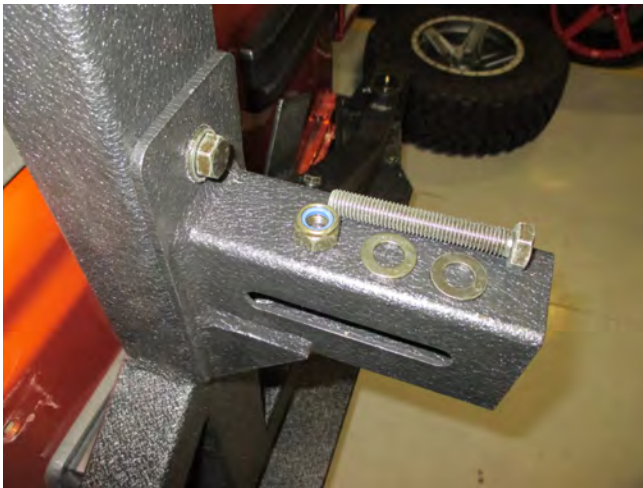
STEP 12 // Install the rear tire carrier and secure it to the rear swing arm at the desired height using the supplied hardware.
