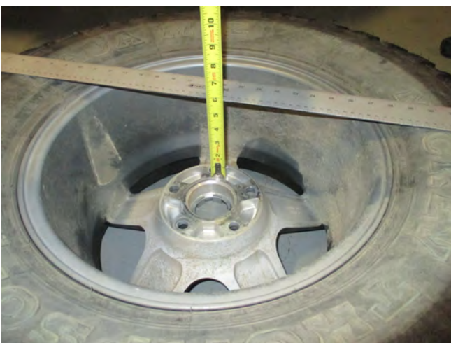
STEP 13 // Measure the backspacing of your wheel and tire by placing a straight edge across the tire. Measure from the mounting hub to the straight edge.
