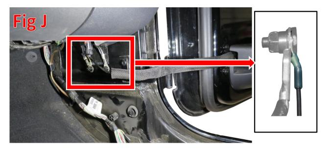
15. Reconnect your battery terminals, open the door, and make sure the dome light and LED Side Step Lights turn on when the door is opened.
