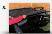
Roll top to rear of the vehicle while keeping top centered on roll cage.
