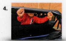
Pull the center back staps to streatch out the top front to back. Check for alignment, tighten straps and stretch top to a tight fit.
