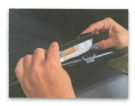
**Step 1:** Connect one of the flat hooks to the tub rail just behind the seat back.
