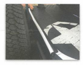
Step 4: Lastly, pull the flap that goes over the tailgate down tight and the magnets will connect.
