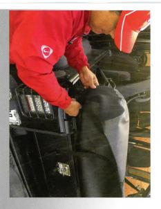
2. Open the tailgate door and loosely slide on the soft top boot over each end. Stretch it over the frame and extend it full length left to right.
