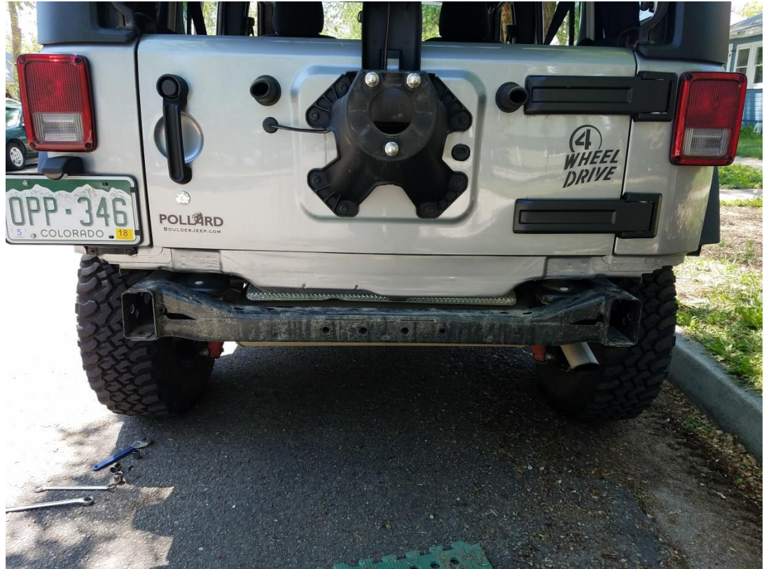
Factory Bumper, brackets and tow hook removed
