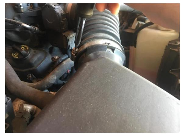
4. Disconnect the temp sensor wire.
