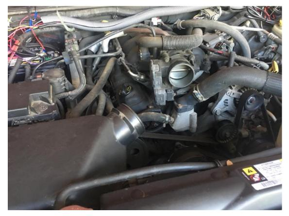
6. Disconnect the crank case vent hose at the back of the air box.
