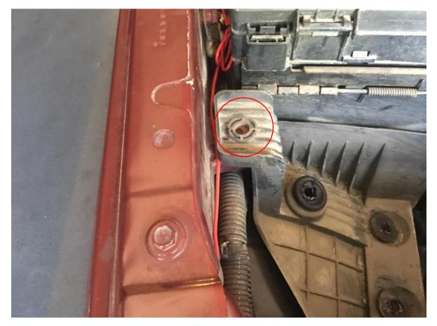
10. Put the trim on the air intake housing, place the housing into the vehicle, and re-install the M6 bolt that was removed in step 9.
