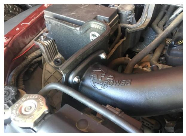
15. Install the crank case vent hose onto the intake tube and tighten the small clamp. Install the filter.
