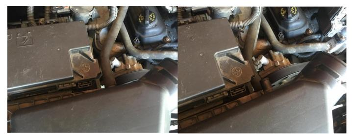
7. Pull the air box straight up to remove it.
