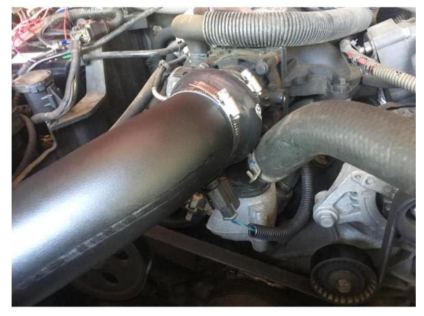
14. Use the provided M6 bolts and M6 washers to attach the intake tube to the housing.
