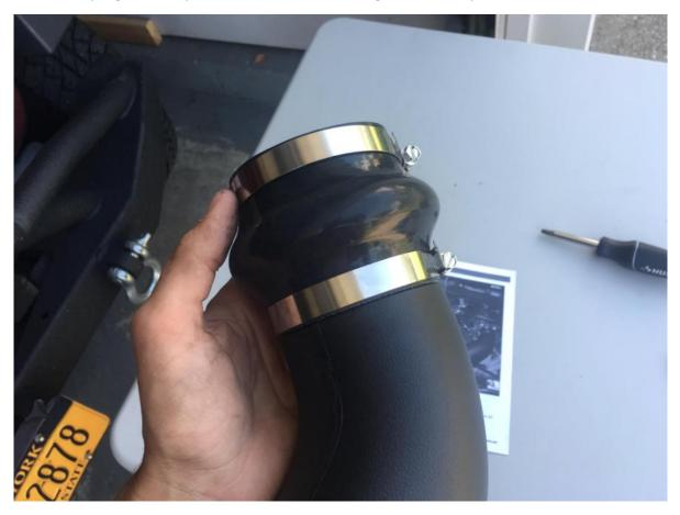
13. Attach the intake tube into the throttle body and tighten the clamps.
