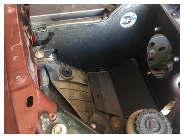
11. Install the aFe grommet for the temp sensor into the intake tube.
