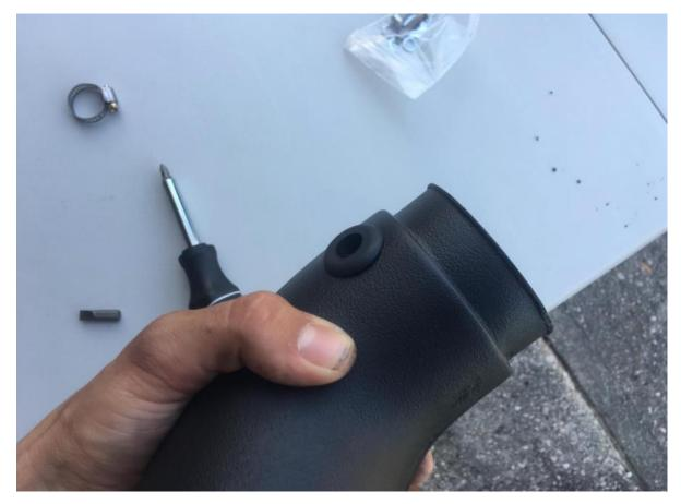
12. Install the coupling and clamps onto the intake tube, along with the temp sensor.
