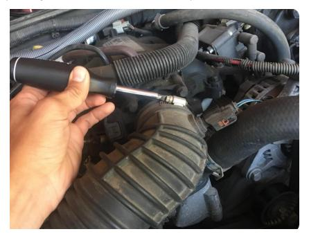
3. Loosen the clamp holding the intake tube to the air box.
