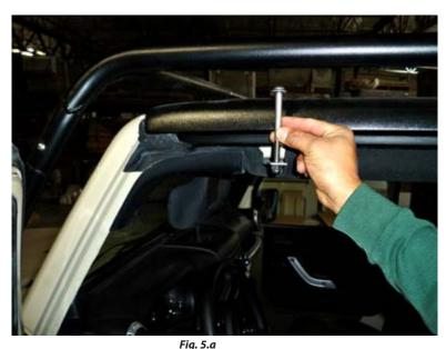
Step 5: Using the two (2) long bolts with acorn nuts and washers that were provided. Drive them in through the top front corners through the rollbar. Use these to tighten down the front corners to your Jeep. (Fig. 5.a)
