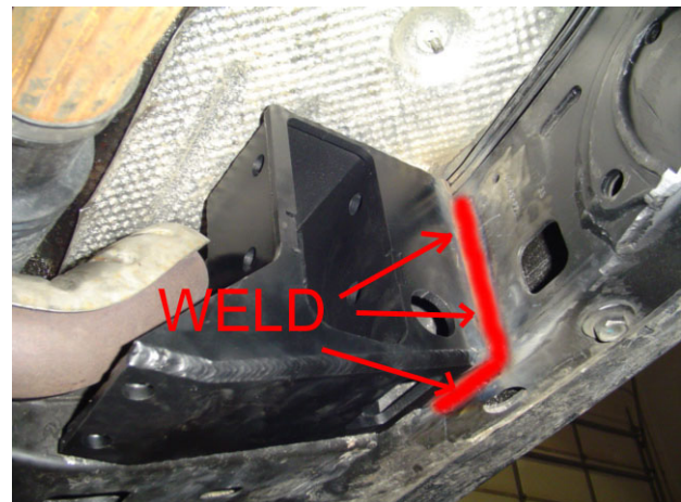
D.S. Bracket Welded in Place
