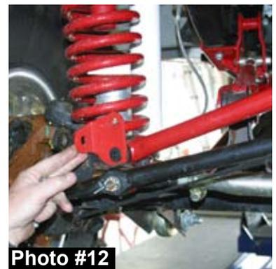
21. Install the frame end of the new Skyjacker track bar by following the hardware pictured. (See Photos # 13 & 14) Being sure to keep the rod end square (parallel) with the frame mount. **Note:** Be sure no more than 1/2" of threads are extended from the bar (including the jam nut). Hold the rod end in place with a crescent wrench & tighten using a pipe wrench or crescent wrench on the jam nut.
