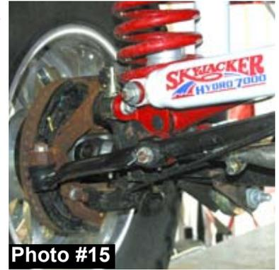
23. Install the front brake lines using the instructions provided with the brake line kit.
