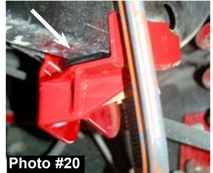
11. Install the new Skyjacker adjustable rear track bar using the instructions provided. Be sure to install both the upper & lower bolts from the rear forward.
