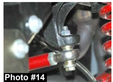
22. Install the steering stabilizer mounting stud in the hole of the drag link & upper mounting hole on the new Skyjacker track bar bracket. Install the provided 5/8 hourglass bushings into the new Skyjacker steering stabilizer & attach to the new Skyjacker studs. (See Photo # 15)
