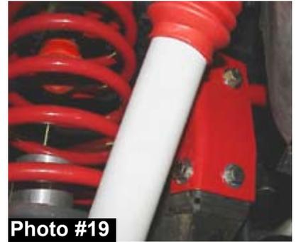
10. Drill a 1/2" hole through the hole in the driver's side of the new Skyjacker track bar bracket. Install the 1/2" x 1 1/4" bolt with washers on each side through the newly drilled hole & tighten with the self locking nut. Install the 5/16" x 1" fine thread bolt, washers, & nut into the forward hole of the new bracket. (See Photo # 19)
