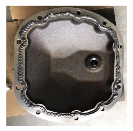
8. Raise the Bombshell cover between the tie rod and the ring gear up into place with the fill plug on the right and start all (10) of the supplied Grade 8 bolts by hand.
