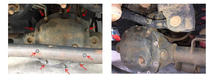
4. Use a razor to cut through a section of the gasket or RTV to begin breaking the seal. Once a small section is open, use a hammer to drive a putty knife between the cover and housing to break the seal. Work around the cover to remove it from the housing.
