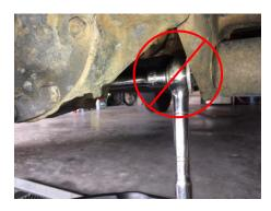
3. Using a  $1/2^{"}$  combination wrench or a  $1/2^{"}$  socket and driver, remove all (10) differential bolts.
