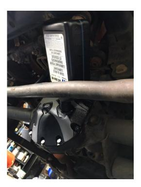
13. Use Teflon tape on the threads of the new fill plug and install to 25 ft-lbs using a short 3/8 in drive extension.
