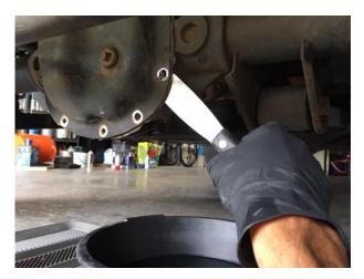
5. Cover gears to prevent foreign material from entering housing and use a razor and wire brush to remove all the old gasket / RTV.
