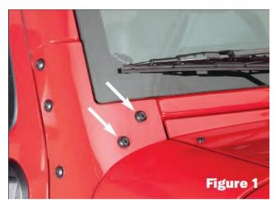
2. Remove Torx Bolts. Using a T40 Torx driver or socket, carefully remove the two located torx bolts. Set these aside for re-installation. **See Figure 2.**
