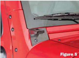
6. The auxiliary lighting can now be bolted onto the light bracket and the wires run under the hood to complete the lighting installation.
