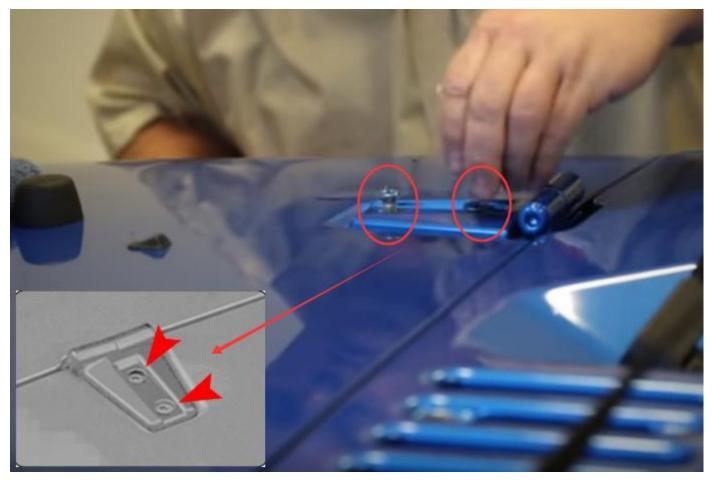
2. Place one of the supplied steel spacers over each hole on top of the hinge, then sit the bracket on top and secure by screwing in the supplied hex bolts + flat washers with the 13mm Socket.
