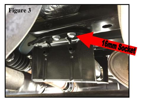
Step 4 – Using a 16mm socket and ratchet, remove the 3 bolts that hold the evap canister in place (2 bolts front, 1 bolt rear). Now you can completely remove the stock skid plate on 2012 and newer models. The evap canister will remain hanging on the Jeep. For 2007-2011 models the mounting bracket will remain on top of the evap canister. (See Figure 2 & 3)
