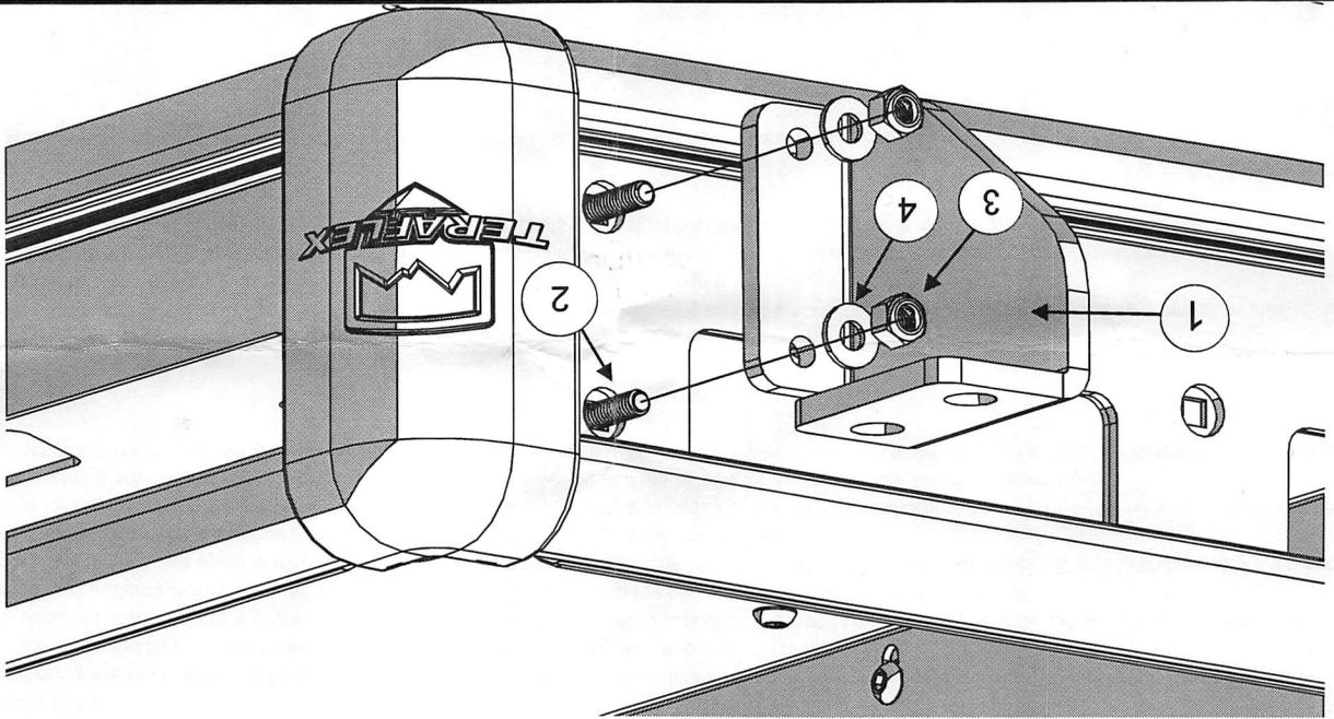
Install the CB Antenna Mount(1) onto the two 1/4" carriage bolts(2). Install 1/4" washers(4) and lock nuts(3) onto the 1/4" carriage bolts. Tighten nuts and torque to 7 ft-lbs (9 N-m). Install CB antenna (per manufacturer's instructions) into one of the top two holes in mount.
