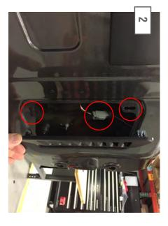
Open the tailgate to access the 3rd brake light connector. Remove the vent cover with a panel removal tool. Unclip the brake light wiring harness. Close the tailgate. Do not install the vent cover.
