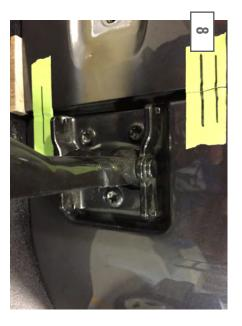
With the hinges unbolted from the tailgate, open the hinge to access the (3) T-50 Torx bit bolts.
