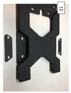
Place the thin spacer behind the upper tire carrier bracket mount, and the thick bracket behind the lower tire carrier bracket mount.
