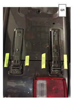
Next, apply painters tape to the vehicle so that you can line up the tailgate correctly if need. Mark the tailgate in several locations. Use a straight edge to mark the tape as a visual reference. Use a razor blade to cut the tape in half at the seam.
