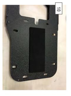
Install the foam cover for the air vent hole. Remove the double sided tape backing on all (4) corners. Install the foam to the tire carrier bracket.
