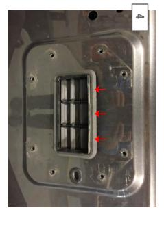
Using a panel removal tool, remove the factory air vent.
