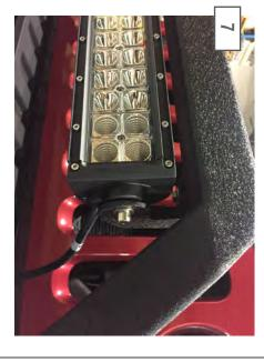
Install the LED light bar using the provided hardware.
