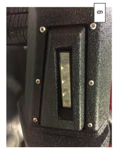
Install the horizontal LED bumper lights. \*\*Note: The mounting tabs may need to be manipulated slightly so that the light can slide in easier.
