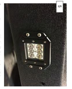
be reused. flush mounted bumper lights. The Allen bolts will Remove the center block off plates to install the
