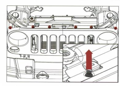
3. Pull bottom of grille away from vehicle to disengage metal clips on bottom rear of grille. Remove factory grille from vehicle.
