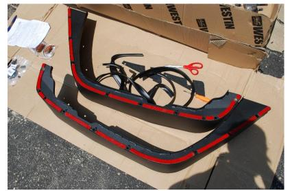
5. Starting at one end of the fender, attach the welting using the double-sided tape. When you reach a bend in the fender, cut small triangles using scissors to allow the welting to bend around the corner and still sit flat on the fender.
