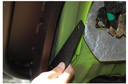
15. Align the front fender and install the 7 6MM hex head cap screws with washers and nuts to attach the fender to the body. At the front of the fender, a 6MM hex head bolt will fasten to the nut in the fender (see photo). Tighten all bolts with the included hex key and the 10MM open end wrench to 10 ft-lbs. Tighten the M8 bolt through the fender support with the 13MM socket to 17 ft-lbs.
