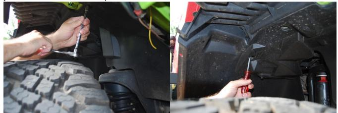
8. Starting at the back of the fender, carefully pull it away from the body of the vehicle. You will hear popping noises as the plastic clips release. The plastic clips often break during removal, but they are not reused with the new fenders. Note that in the picture, the outer fender cover was previously removed, this is not a necessary step.
