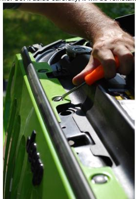
14. Place the fender support behind the body at the rear of the fender and align the bolt holes.
