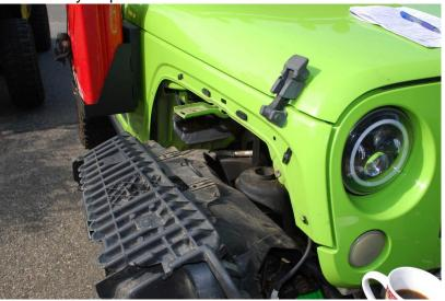
9. Disconnect the electrical connector for the running light.
