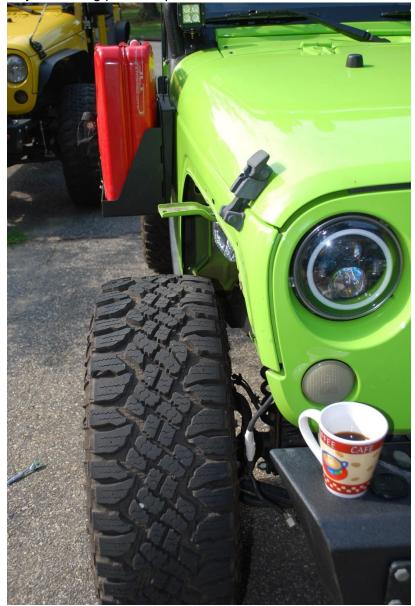
11. Set the new fender on the fender brace and install the included M8 Hex Head cap screw through the fender and brace and attach the included M8 nut. Only tighten it with your fingers at this time.
