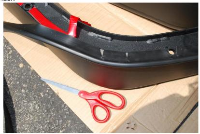
6. Using the X-Acto knife, carefully cut the welting around each bolt hole so the bolts will easily pass through.
