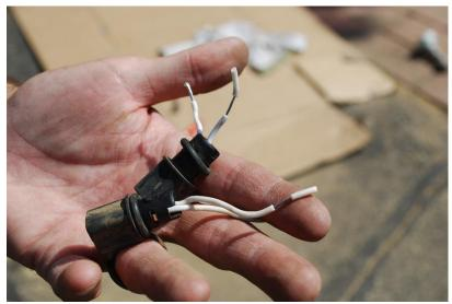
18. Strip  $\frac{1}{2}$  inch of the wire casing from the plugs at attach them to the pigtails for the new turn signals using the soldering iron and solder.
