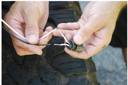
19. Plug the attached pigtail into the factory light harness.
