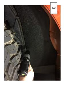
using a 1/8" drill bit. Then drill a 5/32" hole. Mark the remaing holes for drilling. Drill a pilot hole
