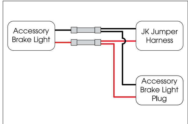
7. Connect Accessory Brake Light plug to factory third brake light harness and connect JK Jumper Harness to factory third brake light.
