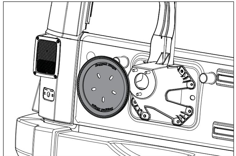
3. Open tailgate. Using T-20 Torx bit, remove four screws attaching third brake light to factory tire mount.
