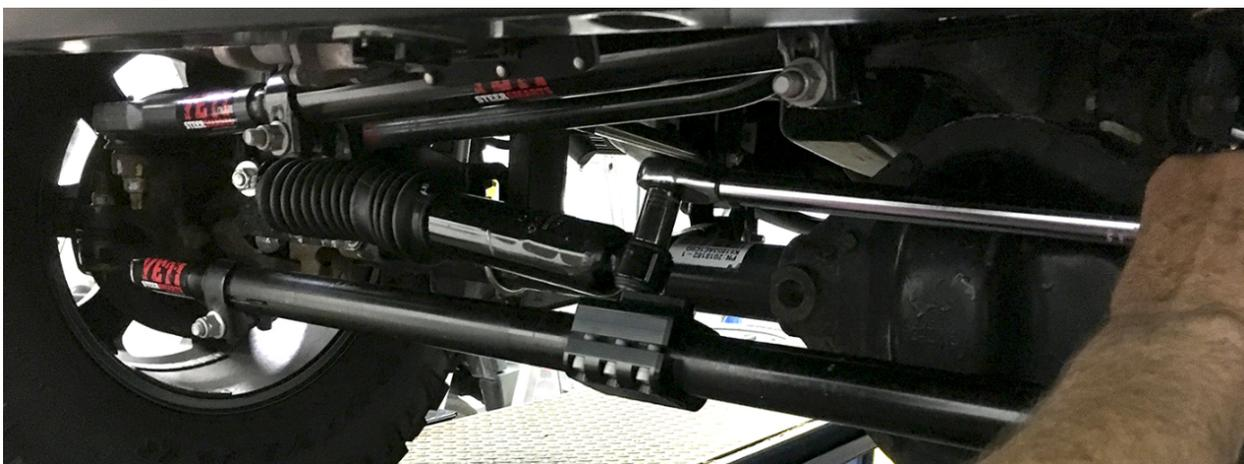
7. Rotate the steering wheel from lock to lock to verify that the damper is centered and does not limit the steering wheel travel. Be sure to confirm that neither the damper nor damper bracket cause interference with other components when being turned from lock to lock.
