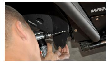
**30. Install a 1/4-20 X 3/4** SS Button Head Cap Screw with 1/4" SAE Flat Washer at each of the three holes that were just drilled in the previous step. Insert the screw into the hole in the inner fender liner, and into the corresponding 1/4-20 U-Nut Clip that was installed in the
