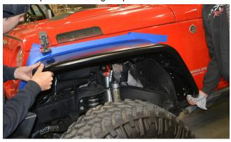
Install two of the  $5/16-18 \times 3/4$  stainless steel flat head cap screws, one at the rear and one at the front end of the Crusher Flare. The one at the front will need to be backed by a flat washer and lock nut (supplied in the hardware kit)
