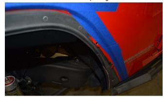
12. Use an auto-punch or a center punch with small hammer to punch a pilot mark into the center of each of the hole marks you made. If you use a hammer and punch, be careful not to strike the punch too hard, as the sheet metal is thin and bends easily.
