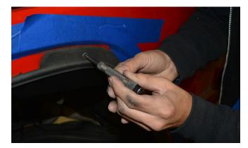
**13. Drill a pilot hole at** each drill mark using a 1/8" bit. Note that two of the hole marks will land on the edge bead of the sheet metal. You must be especially careful when starting to drill these two holes, as the bit will want to walk off of the bead. Hold the drill so that the bit is angled directly into the edge of the bead, wherever it happens to be along the curvature of the bead, in order to prevent walking.
