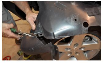
Once the large parts are out of the way, test-fit the inner fender again and make marks for more fine-tuned trimming. It should take several of these steps to finally get it right. Just be sure not to cut away too much in any step, be patient and you will eventually get it just right.
