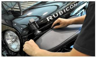
**23. (OPTIONAL) If you are installing** LED side marker lights (sold separately), do so now. Remove the OEM marker light pigtail from the harness, at the plug as shown in the photo. Press on the tang with your index finger, as shown in the photo, to free the plug from the socket while pulling.
