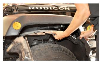
**3. Disconnect the side marker lamp** by pulling the wiring harness plug out of the lamp socket.
