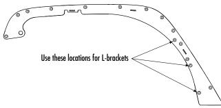
The flat head cap screw should pass through the hole in the Crusher Flare base plate, then through the slotted hole in the "L" bracket (the L-bracket sits behind the flare base plate). The L-bracket should form a 90-degree angle, with the
