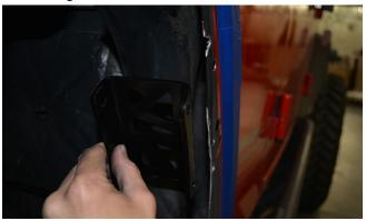
The holes on the Lower Sub Frame Bracket can only align with two specific holes in the outer fender, so position it until you have it properly aligned with the two holes, then hold it temporarily in place by sliding two fasteners from the hardware kit into these two holes.
