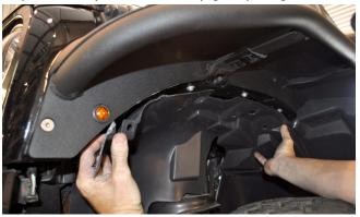
**28.** Once the inner fender liner is trimmed to fit, attach it by first removing the two previously-installed bolts from Upper Sub-Frame Bracket that appear through the access holes in the inner fender liner. Remove each of these bolts, place one of the provided 5/16 fender washers under the head of each, then re-install and tighten.
