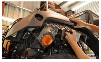
**5. Remove the stock fender flare.** There will be several more plastic retainer clips to remove in order to remove the flare.
