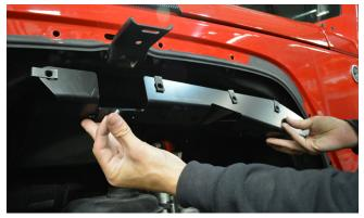
Re-use three (3) of the OEM metric hex head bolts to attach the Upper Sub-Frame Bracket, bolting them through the holes along the bottom of the bracket.
