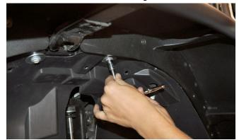
**29. At the rearward edge of** the inner fender liner, mark where the holes in the "L" brackets are located behind the inner fender.
