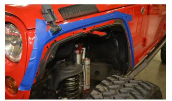
**9. Pre-install the Crusher Flare. Place** it against the Jeep and line up the bolt holes. It will rest somewhat on the stock fender brace to make this task easier. Even with masking tape in place, be careful while handling the Crusher Flare, to keep it from contacting the exterior finish of the Jeep and scratching the paint.
