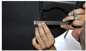
The inner fender liner is flexible plastic, and you will be able to pull it away enough to take your measurements. Mark the hole locations then drill the three holes with a 1/4'' bit.
