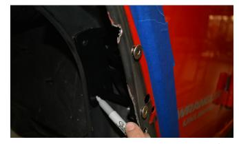
18. Follow the same procedures as in steps 9 and 10 to punch and drill the two holes in the inner tub brace. Drill the 1/8" pilot hole first, then step up to the 3/8" bit. You will have to pass the bit through the hole in the outer fender to reach the inner tub brace.
