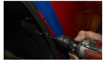
Use touch-up paint to coat the bare metal at the edges of the drilled holes, to prevent rust.
