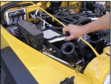
**4.** Remove factory air filter from airbox.
