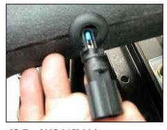
25. <u>For 2005-06 Vehicles:</u> Re-connect the air temp sensor on the backside of intake tube.
