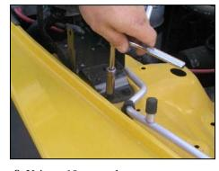
**8.** Using a 10mm socket, remove one bolt from the inner fender as shown above. Retain bolt for later use.
