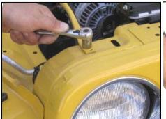
**9.** Using a 13mm socket, remove the radiator rod support bolt on the passenger side. Retain bolt for later use.
