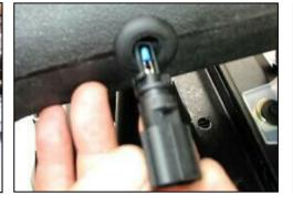
**3.** 2005-06 Vehicles: Disconnect the electrical connector to the air temp sensor on the backside of the factory intake tube and remove sensor. Retain sensor for later use.
