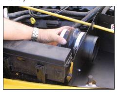
**20.** Install the urethane hump hose and two #72 hose clamps on end of the Airaid Cool Air Dam. Leave hose clamps loose until final assembly.
