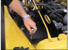
**14.** Using the supplied  $\frac{1}{4}$  x 20 nut, bolt and washers, mount the front of the Airaid Cool Air Dam to the inner fender.
