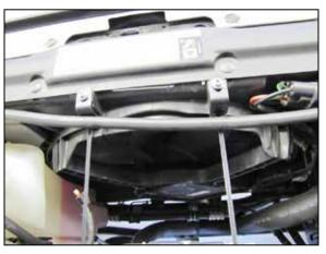
30. Install the tie wrap equipped brackets onto the factory intake tube mounting locations on the fan shroud using the provided hardware. Then secure the coolant over flow hose with the tie wraps.
