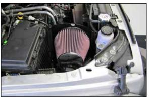
17. Install the K&N<sup>®</sup> air filter onto the filter adapter and secure with the provided hose clamp.
