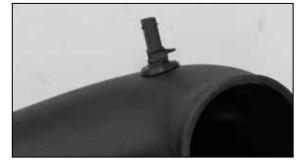
28.Install the provided grommet and factory inlet air temperature sensor into the  $K\&N^{\ensuremath{\$}}$  intake tube as shown.
