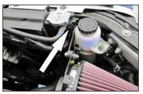
19. Install the heat shield bracket assembly onto the heat shield and radiator mount as shown. Secure the bracket with the factory bolt in step # 9 and the hardware provided.
