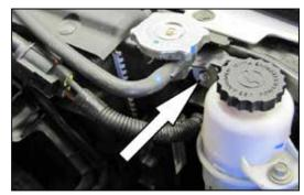
10. Remove the bolt shown that secures the radiator to the core support. **NOTE: This bolt will be reused in a later step.**
