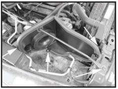
Step 10 Install the heat shield making sure to place the strut thru the cut out in the heat shield. Once in place, fasten it securely in place with the supplied hardware and the hardware that was removed in Step 9.
