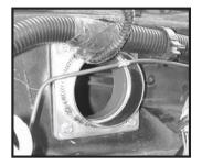
Step 16 Install the supplied firewall duct mount and once it's in place, secure with the four supplied self-tapping screws.
