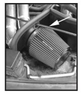
Step 20 Install the filter and securely fasten to the velocity stack adaptor.
