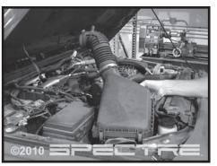
Step 5 Lift up the air box assembly to remove entire unit which is held in place by grommets.
