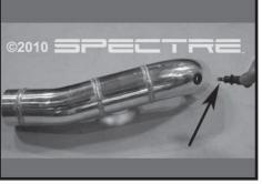
Step 8 Install the supplied grommet into the hole located on the new Spectre intake tube. Reinstall the air temperature sensor into the grommet hole.
