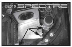
Step 13 Install the heat shield as shown using the hardware that was removed in step 11.
