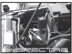
Step 6 Remove the 3 grommets from the factory air box cradle.
