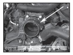
Step 10 Install the coupler over the coupler sleeve on throttle body and fasten securely with the supplied hose clamp. Install a second clamp but do not tighten at this time.
