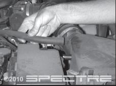
Disconnect the crank case vent hose from the stock intake.
