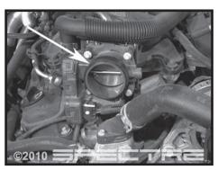
Step 9 Install the coupler sleeve onto the throttle body.
