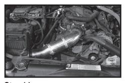
Step 14 Install the air intake tube by passing the filter end through the housing. Align the throttle body end of the tube with the coupler. Once the tube is aligned, fasten securely with supplied hose clamp. (Silicone based lubricants help locate the tube in the grommet.)
