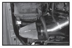
Step 16 Install the Spectre air filter and fasten securely with the supplied hose clamp. Ensure that all clamps and hardware are fully tightened at this time.
