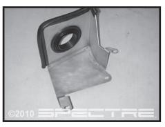
Step 12 Remove the three 10mm screws Dress the heatshield with the 3" grommet and the rubber seal.
