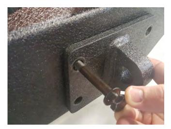
**STEP 7** // With a helper, place the winch mount behind the bumper. Insert (8) bolts and flat washers through the D-ring mounting plate, through the bumper and then through the winch plate. Installing the lock washer and nut on the back side of the frame mounting pad. Ensure all bolts are tight.
