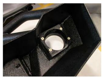
**STEP 5** // Insert the supplied plastic screw retainers.
