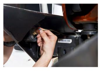
**STEP 8** // In most cases, the fog light harness will need to be extended. Cut and splice the wires to the appropriate length.
