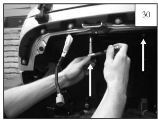
Install a supplied 1.25" Washer on factory bolt/washer assembly and reinstall through factory threads in sheet metal (2 locations).
