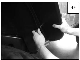
Hold flare in place on fender and start a pan head screw into each hole location and through speed clip on inner structure and metal frame angle support bracket (7 places). Do not tighten.
