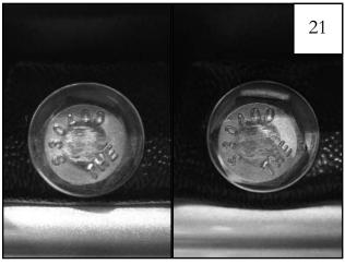
**Bolt on left:** Properly tightened; lower edge of inner piece runs straight
