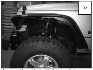
Completed front driver's side flare installation.
