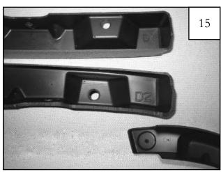
Locate the flat flare front inner pieces. The driver side front inner pieces are marked D1, D2, & D7. The passenger side front inner pieces are marked P1, P2, & P7.
