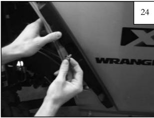
**Step 2** Slide a .700" Washer onto 5/16" Hex Head Bolt. Insert a bolt/washer assembly through inner flare piece and fender and secure with 5/16" Nylok Nut. *Start the bolts but do not tighten.*
