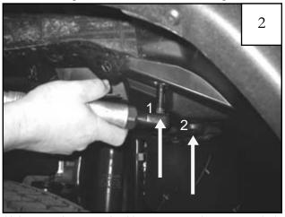
Using a socket wrench with a 10mm socket, remove bolt located in hole inside of splash shield (location 1) and bolt in location 2. Save fasteners for reinstallation. *Note:* 2007-2010 model years have a plastic thread engager in location 2. Remove and save for reinstallation.
