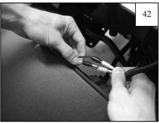
Connect the side marker light wires with the vehicle wires by attaching the male connectors to the female connectors. Test the connection by turning on the front marker/parking lights. Switch connectors if necessary.
