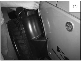
Using sheet metal as guide, mark the rear portion of the splash shield with a grease pencil in preparation for trimming. The splash shield should be flush with the sheet metal after being trimmed. NOTE: If trimmed too little, flare won't fit; if trimmed to much, shield won't stay behind flare.
