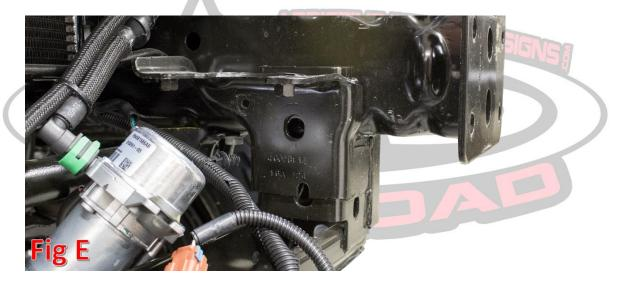
7. Cut off the OEM Vacuum Pump Bracket. We suggest cutting along the weld on the front and back side of the bracket where it wraps around the frame. Once the welds have been cut, the bracket should come off. The area will need to be ground smooth, then painted over. (Fig F)
