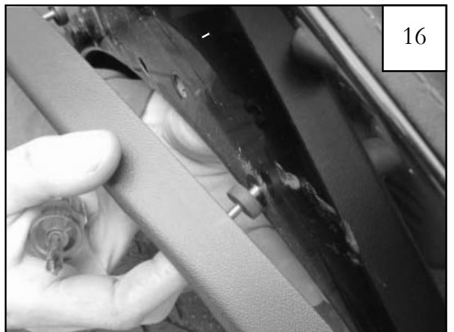
Install inner pieces D2 (and P2 for passenger side installation) to the sheet metal by lining up the M5-.8 machine screws (SW1-0053) with the factory hole locations.
