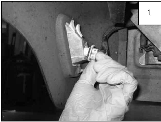
1 Unplug the factory installed side marker lamp by twisting the bulb housing in a counterclockwise direction. This is located at the front of the factory flare on the backside in the wheel well.
