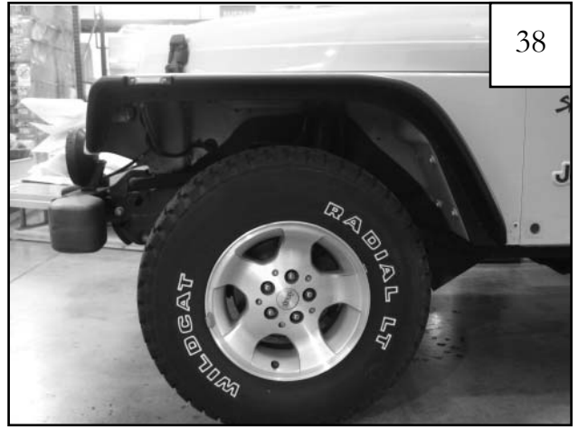
Completed front driver's side flare installation.
