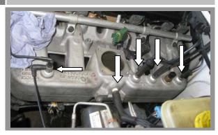
Remove all air lines (6 total) going to the intake manifold.
