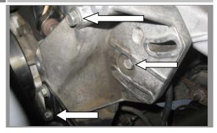
Remove the 3 bolts holding the steering pump bracket to the intake manifold.
