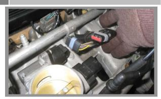
Unplug all the electrical connections going to the throttle body. Unbolt and remove the throttle body.
