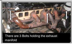
Remove all the hardware and remove the stock exhaust manifold from the vehicle.
