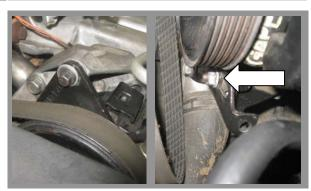
Remove the top bolt on the black bracket above the pump and the nut on the bottom of the steering pump.
