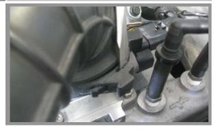
Loosen the clamp at the throttle body by pulling the locking tab up.
