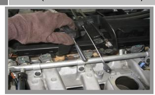
Unbolt the bracket holding the throttle body cables and move to the side.
