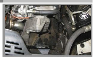
After removing the belt and un-mounting the steering pump, move it off to the side to aid in Header installation.
